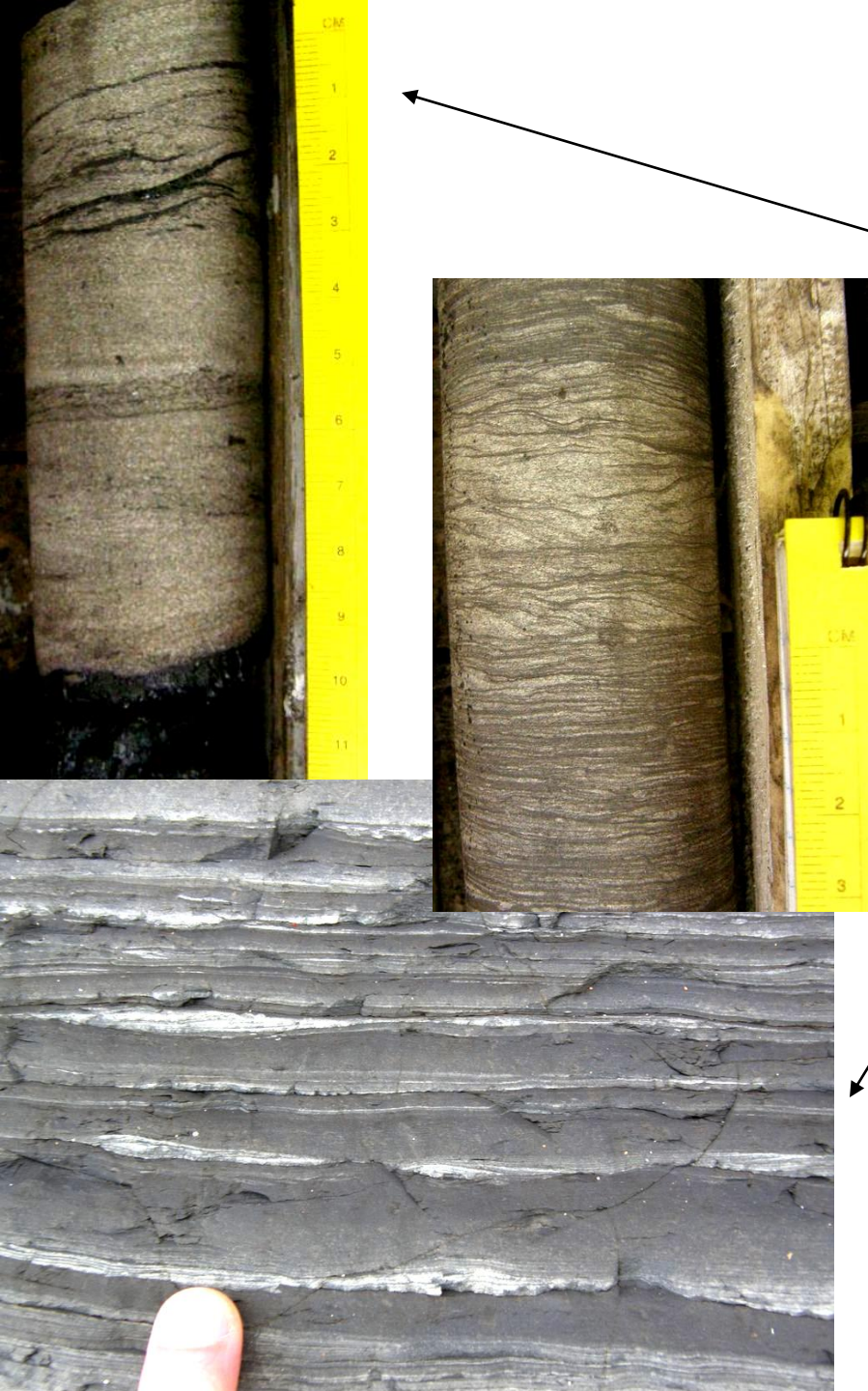
Fig. 4.25 Mixtures of sand and mud in different proportions produce different forms of lenticular and wavy bedding. (After Reineck & Singh 1973.)
