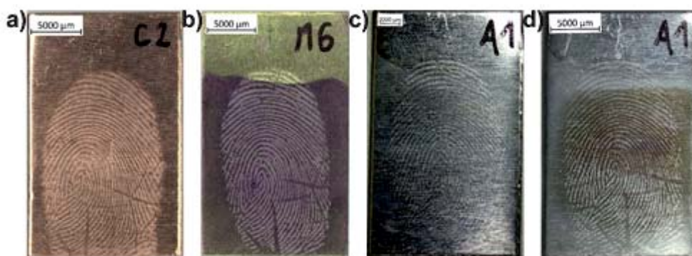
Fig. 1 Visualization of fingerprints using Britton-Robinson buffer: a) copper at pH = 7, b) brass with methylene blue at pH = 7, c) aluminium at pH = 2, and d) aluminium at pH = 2 after 5 days.
