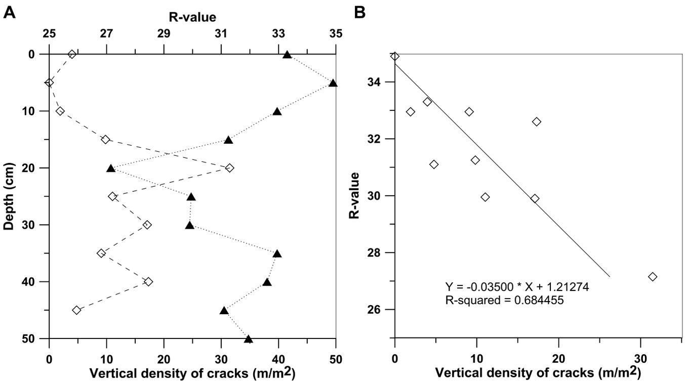
Figure 7. R-values and density of cracks versus depth at Site 20. Solid and unfilled shapes represent Rvalues and cracks, respectively.
