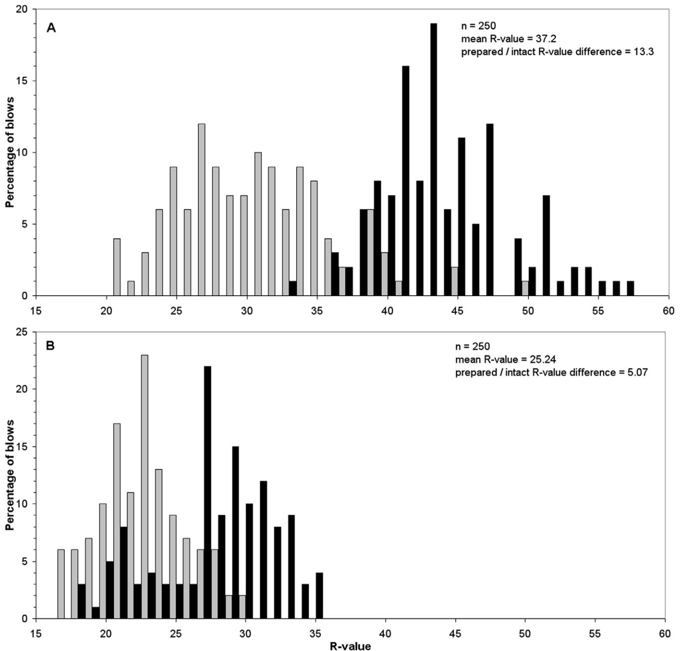
**Figure 8.** Frequency distributions of Schmidt Hammer single impacts for relatively fresh (A) and weathered (B) surfaces, represented by roches moutonnées and tors above 560 m a.s.l., respectively. Grey bars represent data from natural surfaces and black bars represent prepared surfaces.
