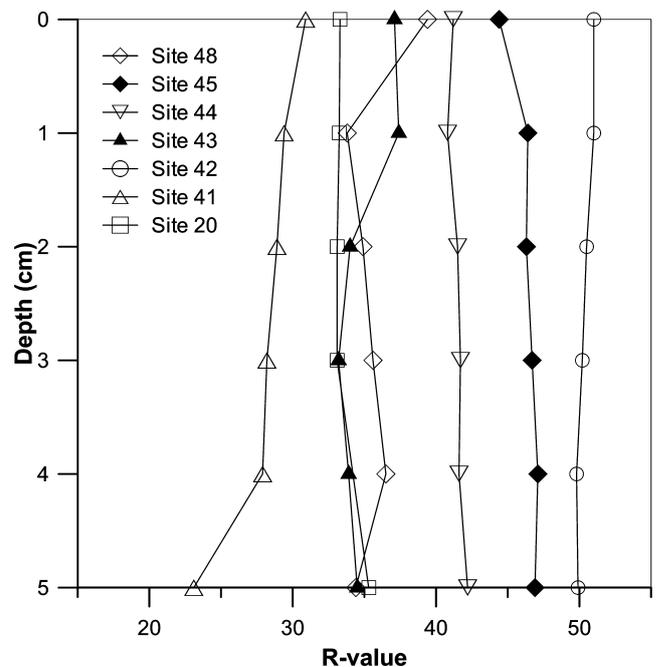
Figure 5. R-values down to 5 cm depth. Solid and unfilled shapes represent coarse- and medium-grained granite, respectively.
