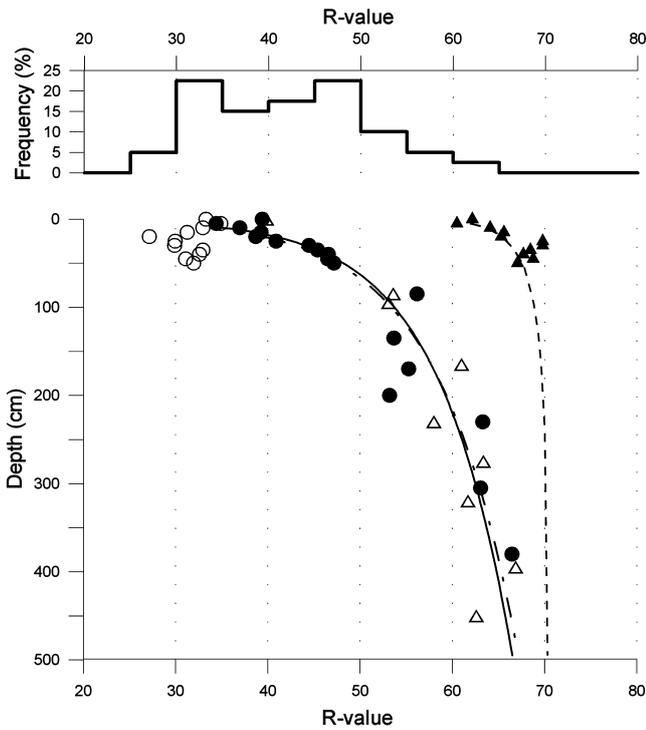
**Figure 9.** Depth versus R-value plot for vertical profiles and step plot of R-value frequencies measured on prepared surfaces in the study area. Solid triangles, dashed fit – Site 47 (river channel); solid circles, solid fit – Site 48; unfilled triangles, dashed and dotted fit – Site 46; unfilled circles – Site 20.
