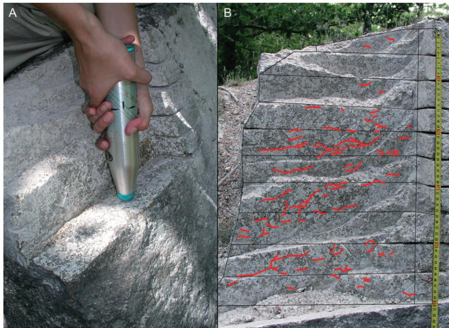
**Figure 2.** SH applied to horizontal surfaces along 50 cm deep vertical profiles (A). Vertical cuts with marked cracks (B). This figure is available in colour online at [wileyonlinelibrary.com](http://wileyonlinelibrary.com)
