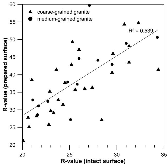
Figure 4. R-values on prepared versus intact surfaces.
