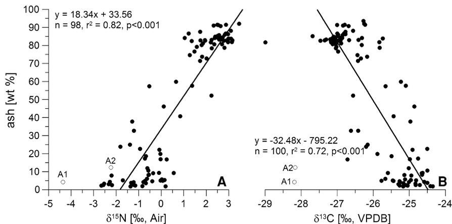
**Fig. 7** Relationship between ash content (wt%) and  $\delta^{15}\text{N}$  (a) and  $\delta^{13}\text{C}$  (b) for all samples. Isotopic composition in the pure peat layer (ash content <10%) varies within a wide range compared with the samples of other sediments having ash
